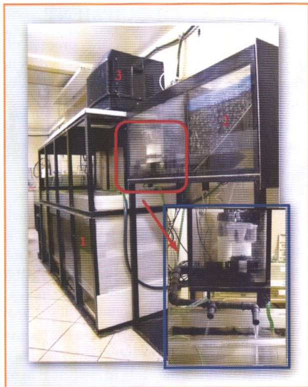
Figure 34. Fragment of a recirculation system (VNIRO, Moscow): 1 – Holding tank; 2 – Biofilter; 3 – Chiller.
